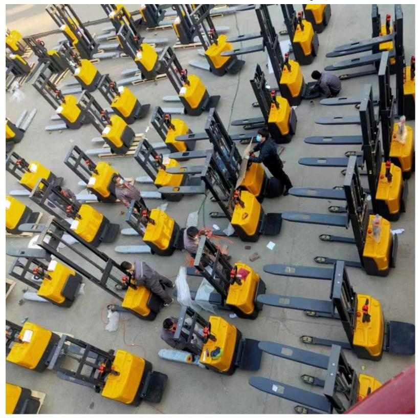
Walking type electric pallet stacker are self propelled pedestrian controlled electric power stacker, with electrically operated lifting function. The trucks are designed for stacking operations in dedicated racking by lifting and lowering the palletized load up to the desired lifting height.
